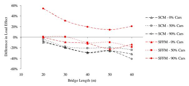
Figure 3 – Impact of traffic microsimulation on load effect.
