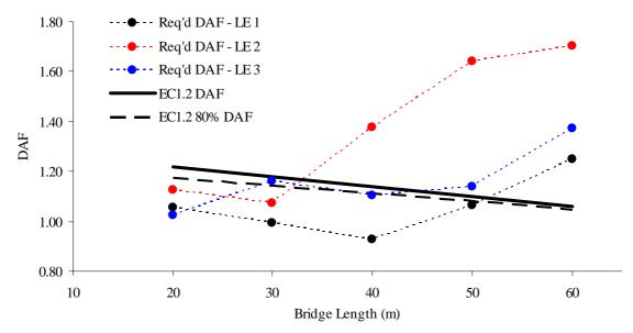
Figure 4 – Identification of governing traffic state through required DAF.
